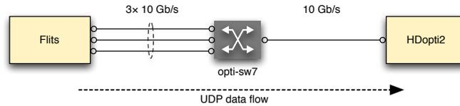
**Fig. 8.** Triple network link configuration between two hosts. Since UDP is used, the data is dropped at the switch.
