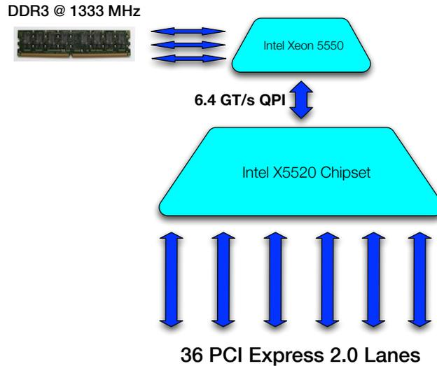
Fig. 1. Typical architecture of an Intel Xeon 5550 and 5520 chipset.
