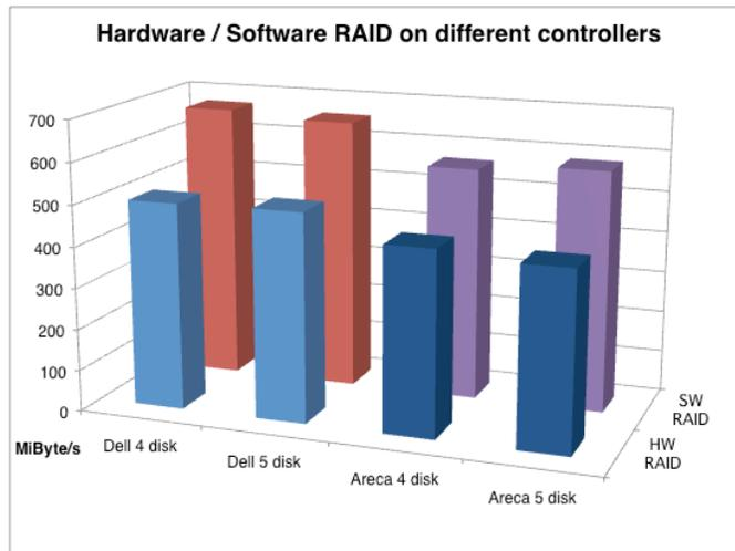
Fig. 6. Comparison for hardware and software RAID.
