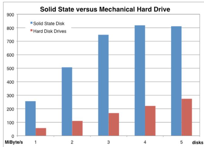
Fig. 2. Disk array read performance for up to five solid state disks.
