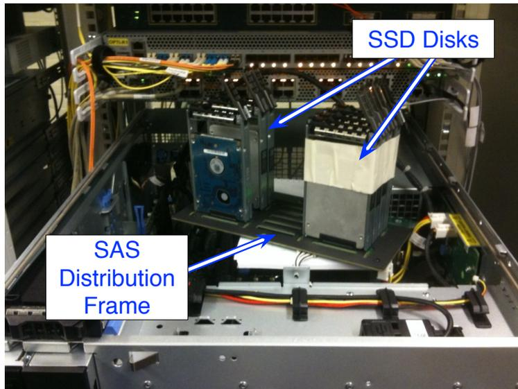
Fig. 4. Experimental setup with the RAID controller in a PCI Express 2.0 slot.
