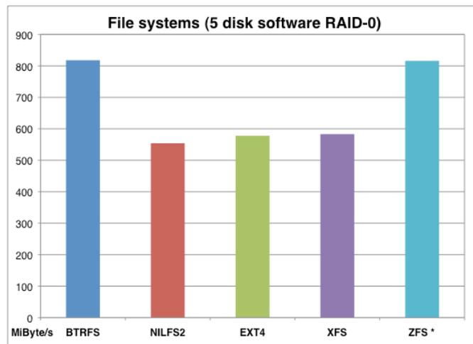
**Fig. 5.** Read performance with different file systems. ZFS runs under FreeBSD, the other file systems under Ubuntu Linux.
